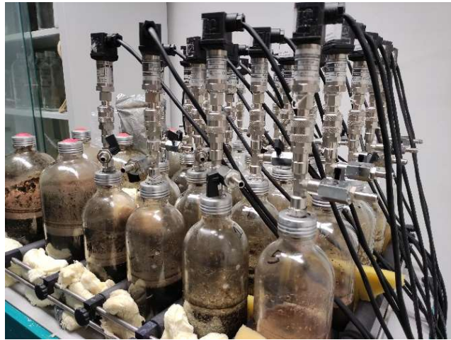
Figure 2. Lab setup for monitoring VFA production from waste streams.
