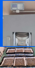
Figures 2a,b: Images from the compression test of concrete samples and freeze-thaw by exfoliation
