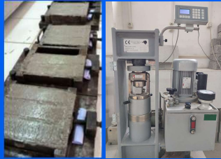
Figures 1a,b: Images from obtaining and testing compression mortars
