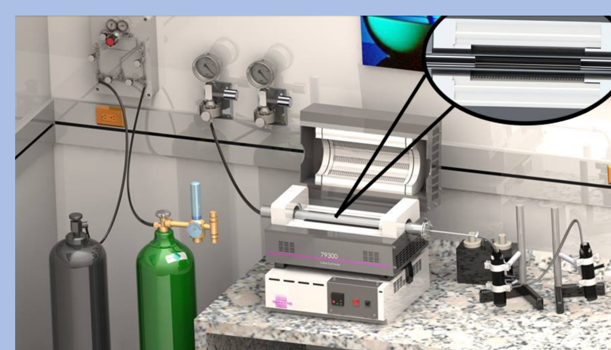
Fig. 1a. Oven to prepare activated carbons from cashew nut shell waste solids, under inert atmosphere.
