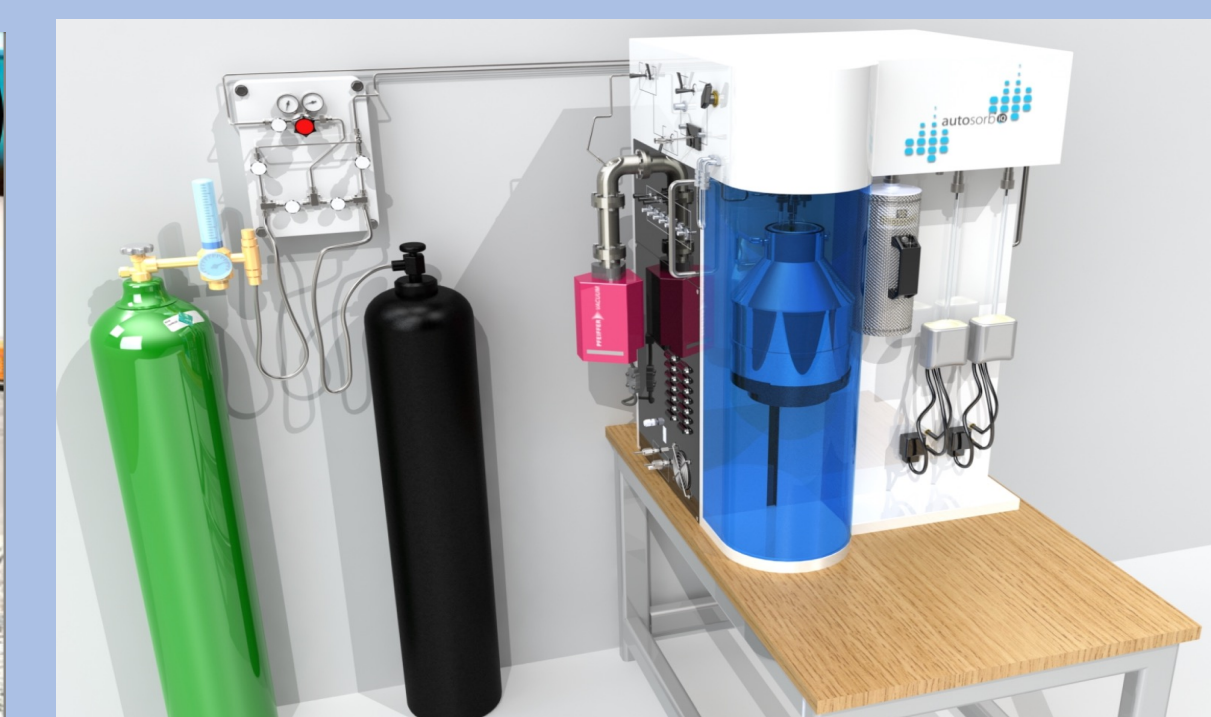
Fig. 1b. Sortometer for measuring N 2 adsorption isotherms at 77 K.
