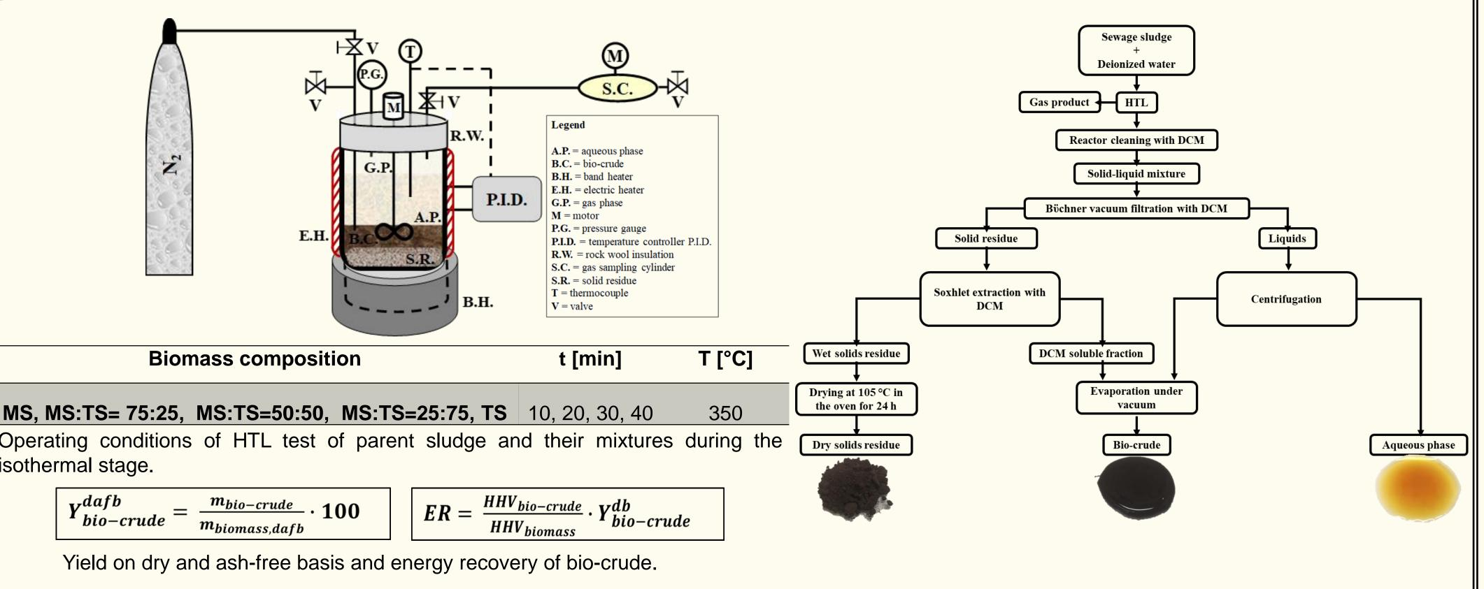
The average yields of bio-crude on dry and ash-free basis show a synergistic effect for the mixtures compared to single sludges.
