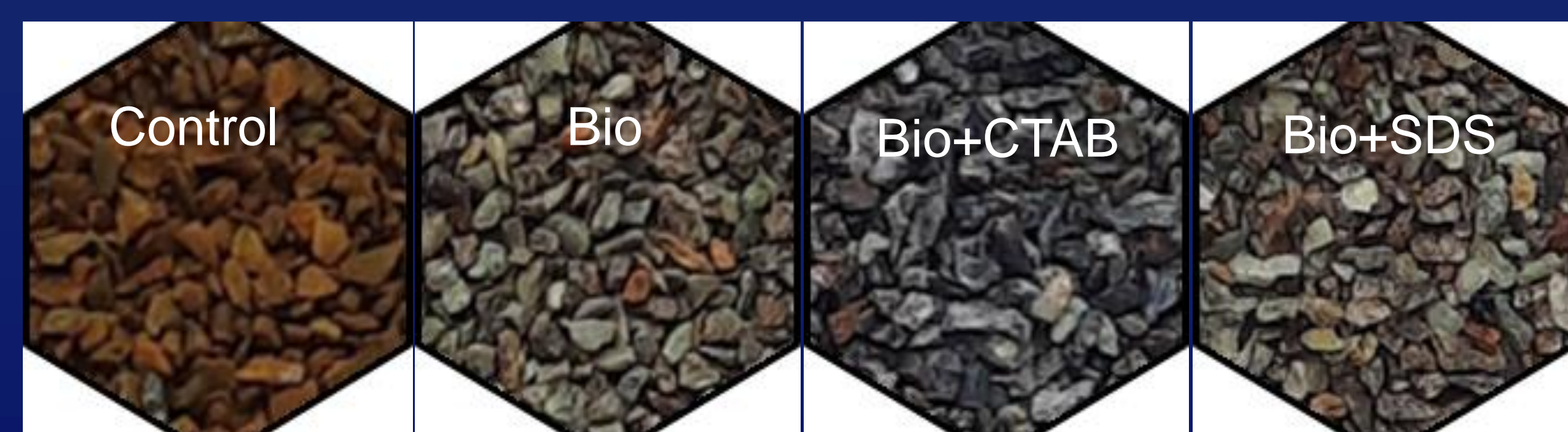
Figure 3. Mineral particles of arsenic waste after bioleaching
