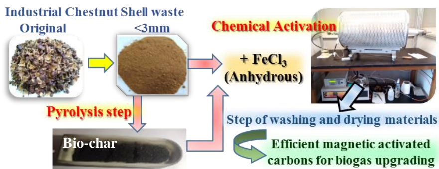
Fig. 1. Preparation of magnetic activated carbons from industrial chestnut shell waste or its bio-char.
