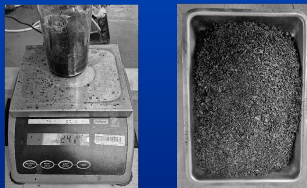
Figure 3. Examples of pyrolysis products obtained from the MDF sample: pyrolytic oil and char
