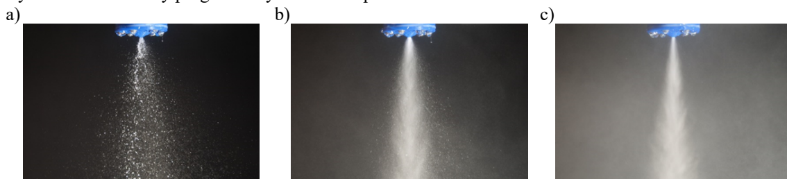
Figure 2. Visualization of the spray for liquid flow rate 20 l/h: a) gas flow rate 1 m 3 /h, a) gas flow rate 3 m 3 /h, c) gas flow rate 5 m 3 /h.
