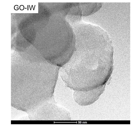
HRTEM visualization of GO-IW indicates the presence of few layer graphene material with low lateral size
