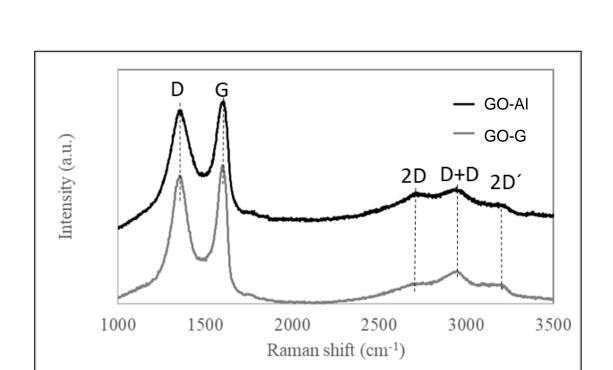
The Raman spectrum of GO-Al shows the typical shape of a graphene oxide, very similar to that of G-GO (from standard graphite). The ID/IG ratio obtained for GO-Al is 0.95, a bit lower than that calculated for GO-G (0.97).
