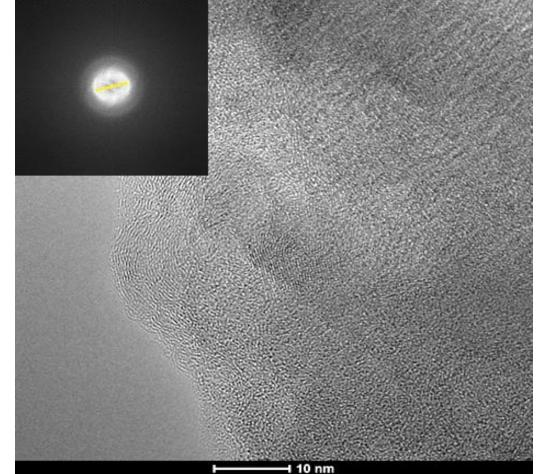
The appearance of more wrinkles and defective edges in GO-Al is noticed by means of HRTEM visualization, in a similar way to other graphene oxide sheets from biomass sources
