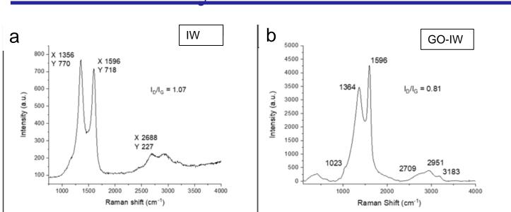
The ID/IG intensity ratio for the raw industrial waste (IW) is of 1.07, in accordance with a poor graphitic structure. However, after processing, the ID/IG ratio of the GO obtained without graphitization is of 0.81 in the range of a standard graphene oxide (GO-G, 0.97).
