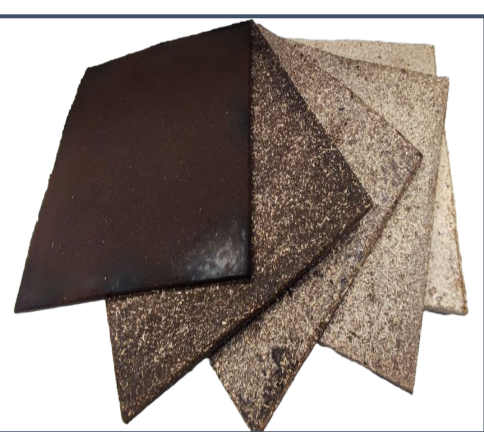
Figure 2. Particleboards with different concentrations of coffee grounds.
