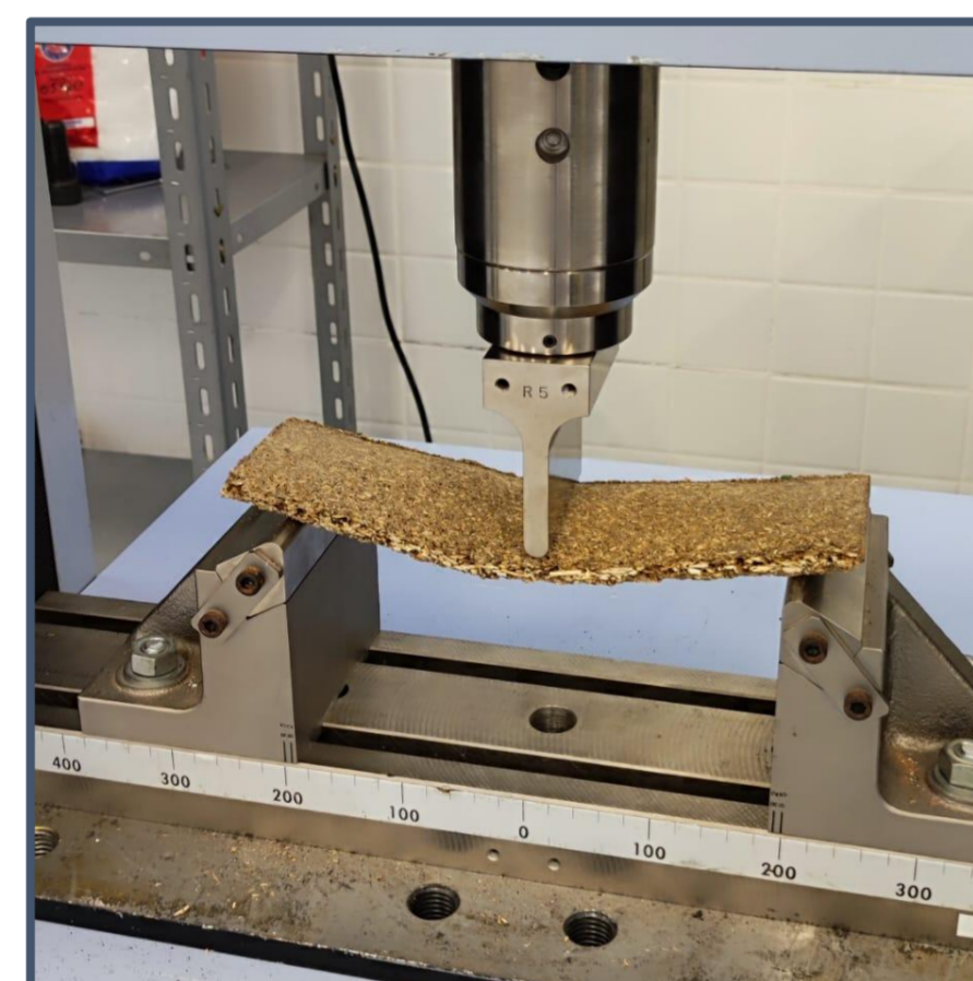
Figure 3. Flexure test of 50C-50W-15UF-3L-4C-6S specimen
