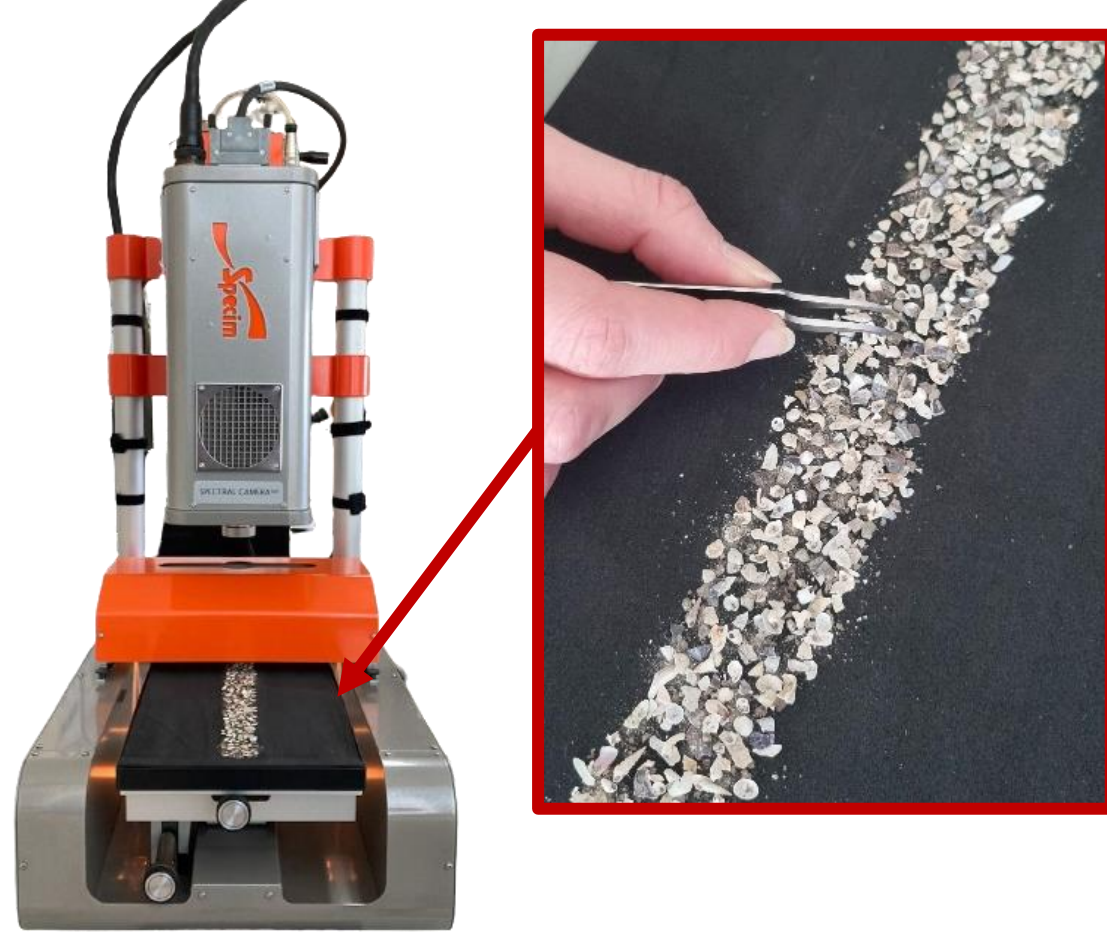
Fig. 3. HSI acquisition platform used to acquire the examined marine sediment samples.
