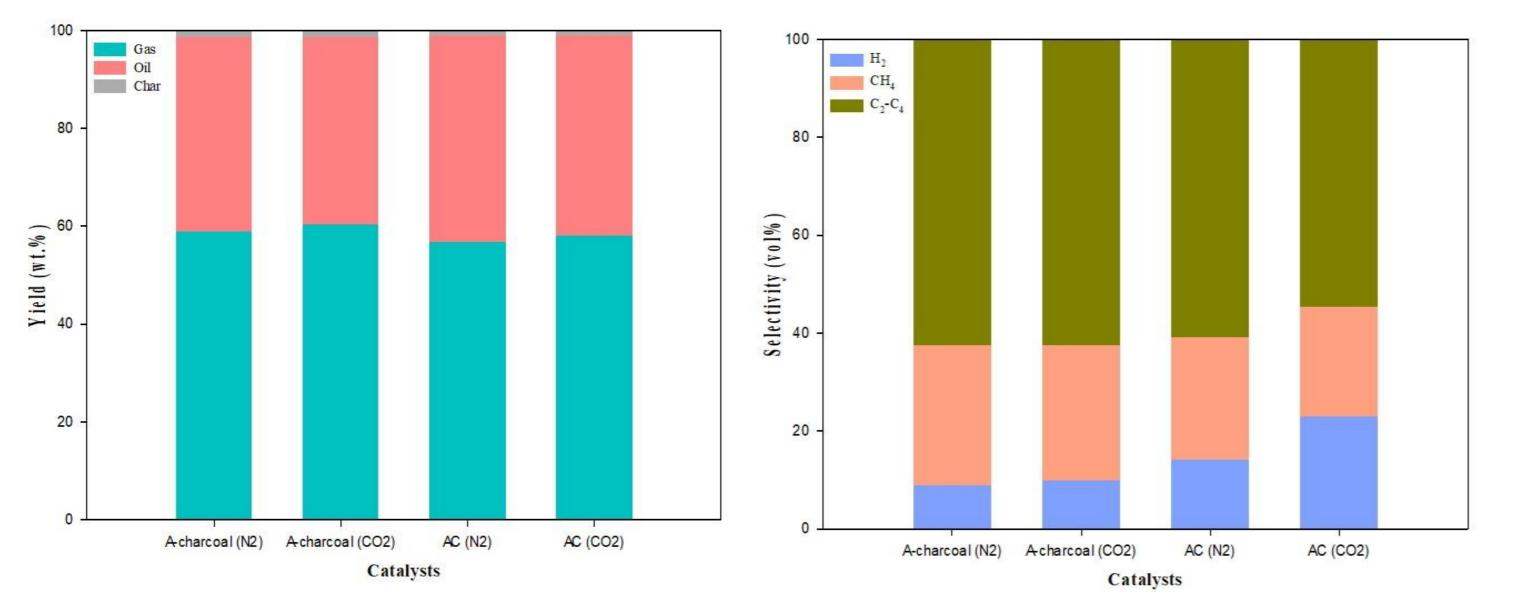
• Disregarding catalyst and environment type, yield of different products did not change considerably. In the case of activated carbon, H<sub>2</sub> selectivity increased under CO<sub>2</sub> (22.94 vol%) than under N<sub>2</sub> (14.09 vol%).
