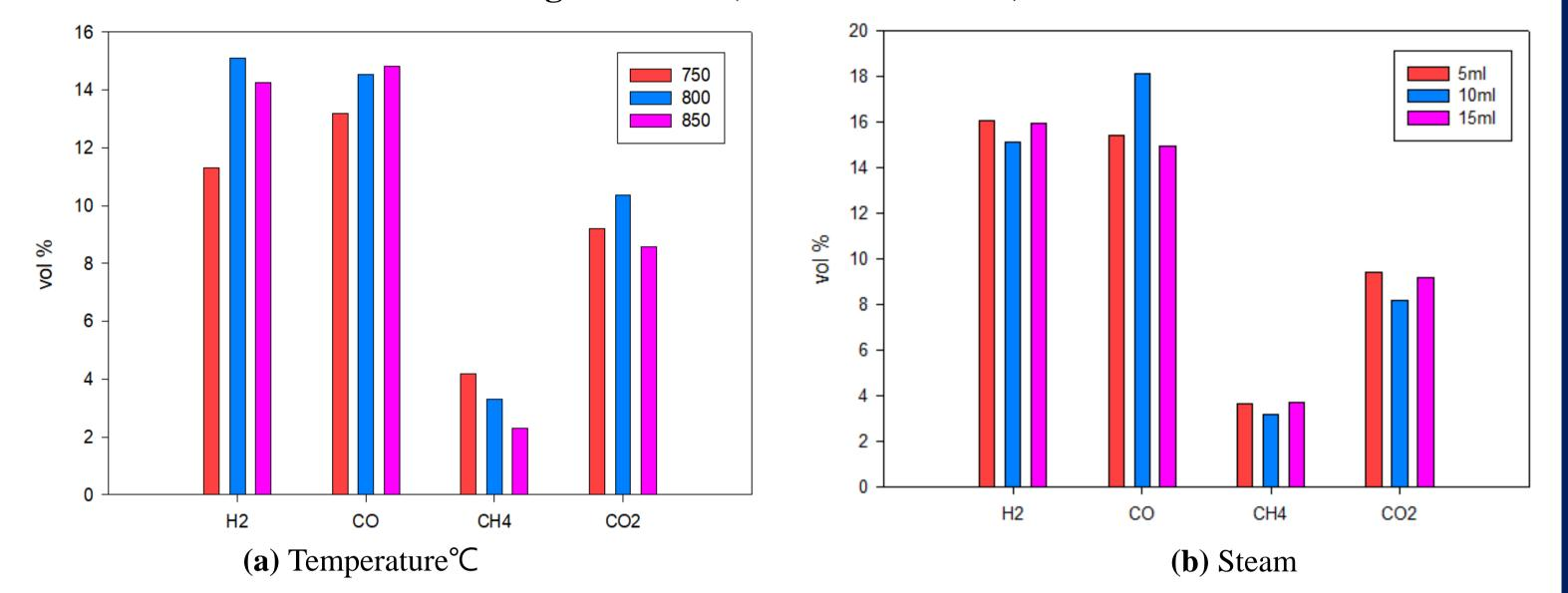
Effect of air/steam injection and reaction temperature on gas selectivity of DSS gasification(Bio char)
